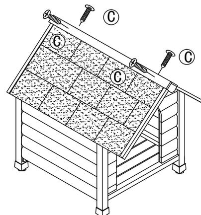
step 4 : secure the ridge cap to the roof with scews C.
